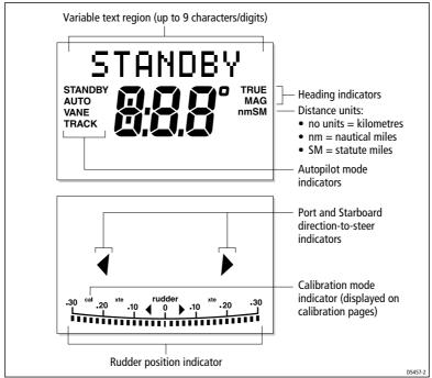
The bar graph at the bottom of the screen indicates the current position of the rudder, as measured by the rudder position sensor.
